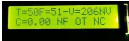
Figure 15: Over temperature output
